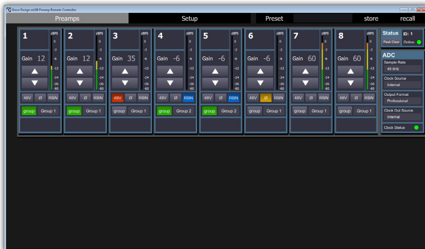
The m108 can be controlled remotely via a Windows/OS X application or a web page.
