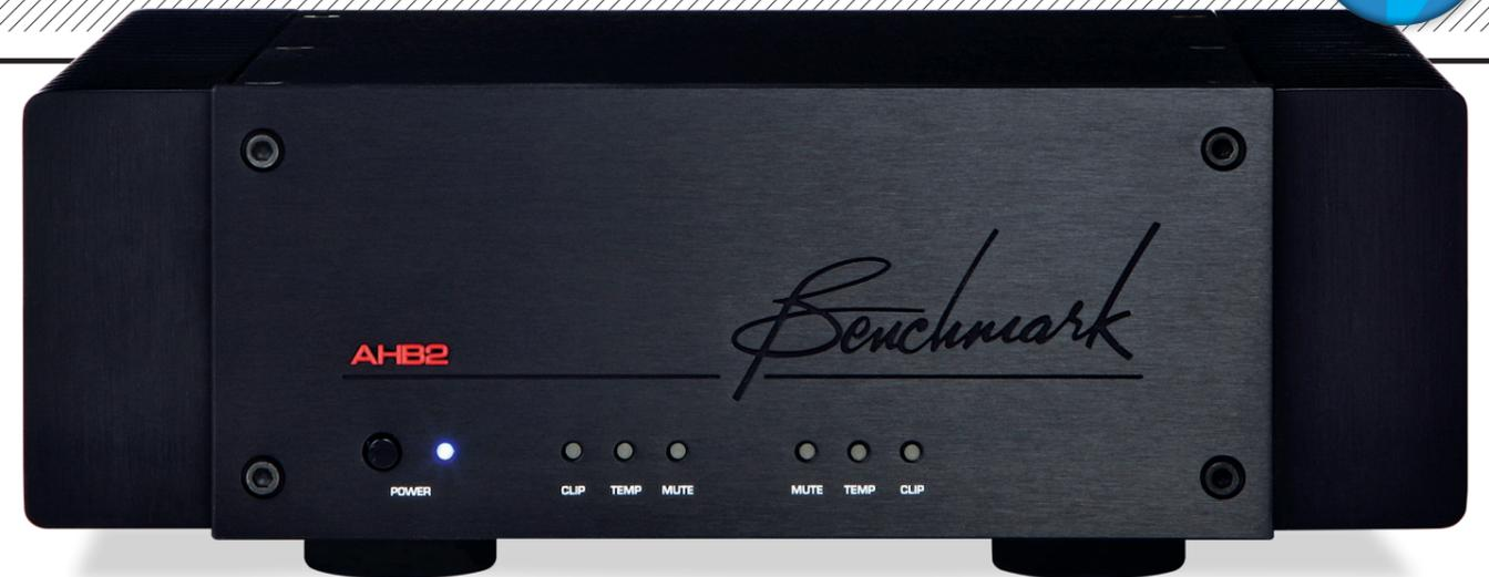
result is said to be an amplifier with Class A-like characteristics, including freedom from crossover distortion, and the ability to run the output devices with very low bias, thus reducing waste heat and power consumption. Key to all this is the THX-patented 'AAA' technique that employs a feed-forward error correction amplifier running in parallel with a higher-power main amplifier.
