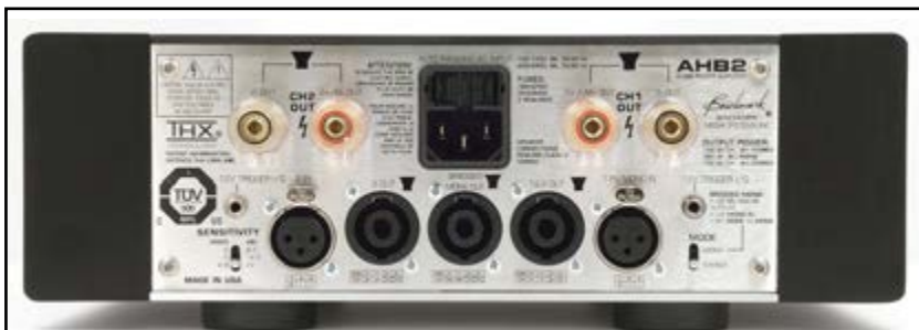
Photo 6: The AHB2's rear panel shows the balanced XLR input jacks, Neutrik SpeakON connectors, and gold-plated binding posts for loudspeaker connections, 12-V Trigger I/O, and the IEC power connector. The three-position gain and stereo/mono switches are on the lower left and right. (Photo courtesy of Benchmark Media Systems, Inc.)
